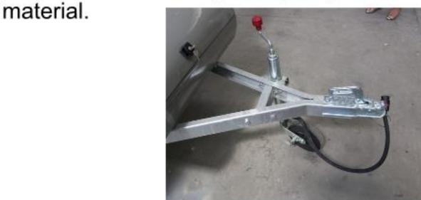
■The connection plug is 13 pin socket which enables charging the trailer 's battery throught the car battery and functioning the 12V powered units, beside enables the signalization. 13 pin is arranged based EU Standard.
